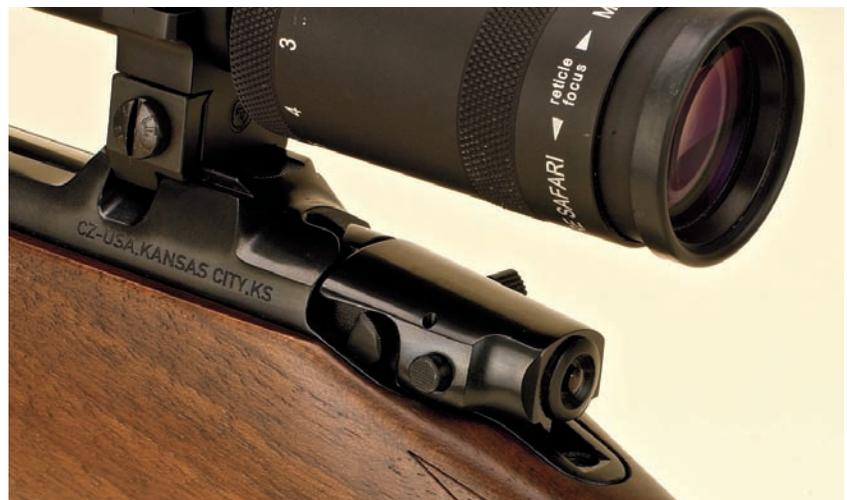
A bolt release and bolt disassembly catch on the left side of the gun make maintenance easy.
